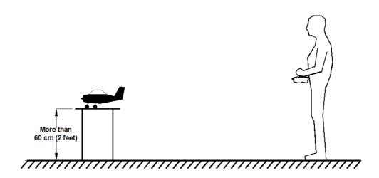
Human bodies absorb radio energy, so if, instead, the model is being held by someone they should hold it away from themselves and keep their body from the path of the signal. Take care others do not stand between yourself and the model. Make sure the ground is flat or has a dip over the area you are using. Even a shallow hump can obstruct the signal.
