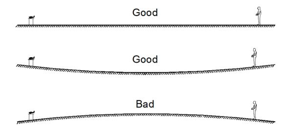
We have said that the body absorbs radio energy and obstructs the signal. When doing the test you must face the model. Walking backwards across a field is often not a good idea so I normally walk about ten paces at a time before turning to check operation then count my steps when walking back to the model once the limit is reached. I know my stride is about a yard (90 cm), and consistent enough for such tests. You will need to check your own stride length.
